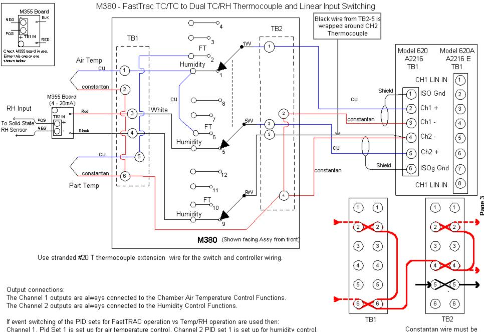
Channel 1, Pid Set 1 is set up for air temperature control, Channel 2 PID set 1 is set up for humidity control.
