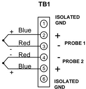
Type T Thermocouple shown
