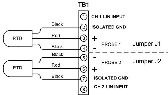
Note: For 2 wire RTD's install a jumper between pins 2 & 4, ( 5 & 7 )
