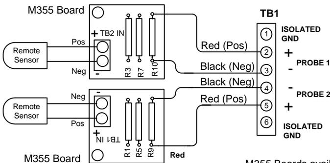
Two different M355 boards are supplied for the units. Make sure the board in use is hooked up properly.
