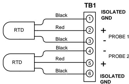
Note: For 2 wire RTD's install a jumper between pins 1 & 3, ( 4 & 6 )
