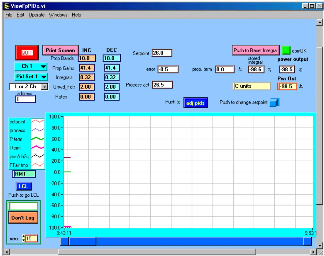
This screen allows visual access to the Proportional action, Integral action, Power output % while showing the effects of each of the above on the Process vs. the Setpoint. It speeds up dramatically the tuning of the controller. A data log capability is provided to allow records of chamber performance and controller internal actions in real time.
